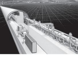
Two particle detectors will be placed at the point of collision and takes detailed measurements at the very moment of collision. The ILC uses two different types of detectors.
